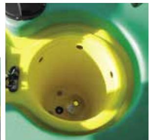
**Premixer:** for the preparation of the chemical mixture both with powder and liquid. An automatic system allows the emptying of "Premixer" without any inhalation or contact with the operator.
