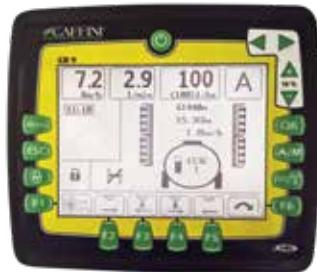
**Computer CB9** for the automatic control of the treatment. The display shows l/ha during the treatment, the sprayed liters, the treated area.
