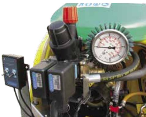
**Motorized compensated valves kit Compact** composed by 2 electric valves for the distribution on left and right side, pressure adjustment on the pump, self-cleaning filter and manometer Ø 100 mm.
