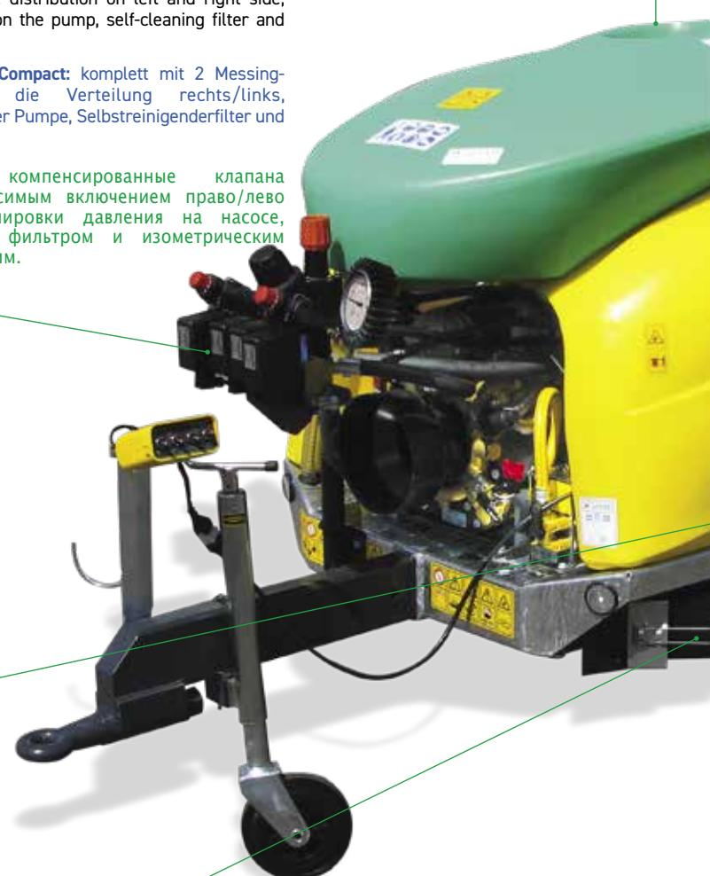
The **distribution pipes** under the frame are in stainless steel (no maintenance). Frame and fan group are hot galvanized.
