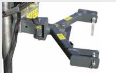
Steering drawbar with tractor lower arms linkage.
