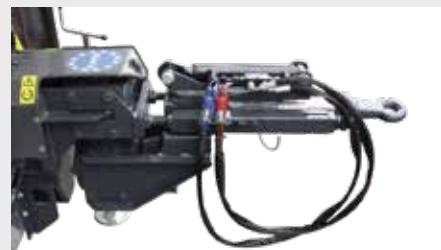
Draw bar with gear steering transmission.
