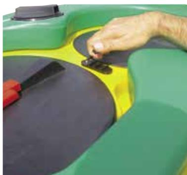
The **emptying** from the top side through a cord avoids all the contacts of the operator with the chemical mixture.
