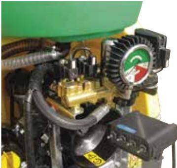
**Electric Valve kit** composed by 2 electric valves in brass for the distribution on left and right side, and pressure adjustment on the pump. Self-cleaning filter in stainless steel and manometer Ø 100 mm complete the equipment.
